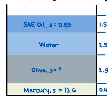
Gage pressure at the bottom of the tank:  $P_{gage} = 231.3 - 101.3$ = 130.27 kPa
