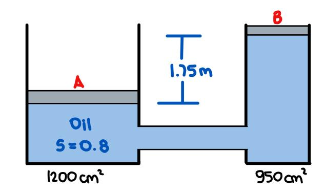
18. Determine the weight W that can be carried by the 1.5 kN force acting on the piston.
