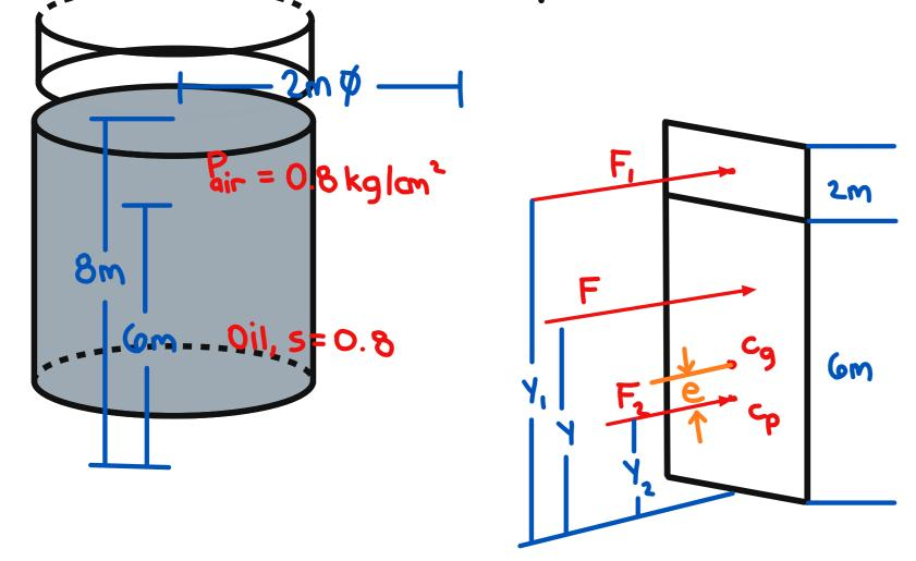
$$\frac{0.8 \text{ kg}}{\text{cm}^2} \times \frac{10000 \text{ cm}^2}{\text{m}^2} = 8000 \text{kg/m}^2$$
