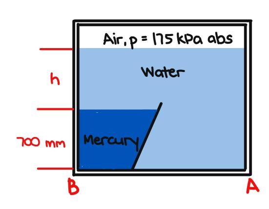
Pressure Head at B to  $P_2$ .  $\frac{P_B}{Y} - 0.7(13.6) - h = \frac{P_2}{Y}$   $\frac{290}{9.81} - 9.52 - h = \frac{175}{9.81}$  h = 2.2 m
